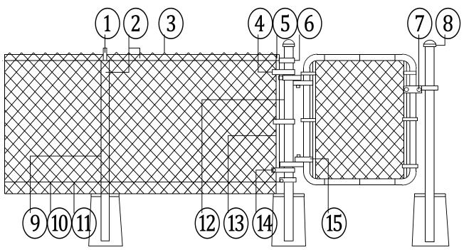
Fittings for chain link fence assembled with gate
